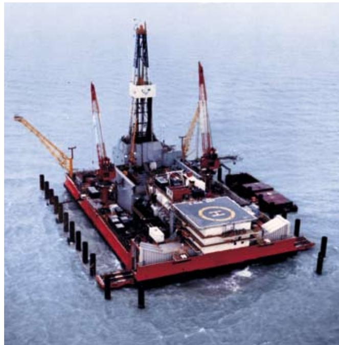
The *Sunkar*, or Parker Drilling barge rig 257, was designed and constructed in New Iberia specifically for drilling the North Caspian Sea's giant discoveries and is the world's only arctic-class barge rig in operation today.
